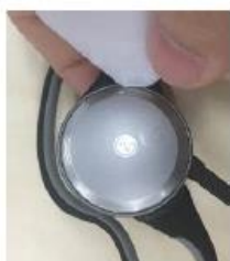
Using a tool, detach Upper case.
