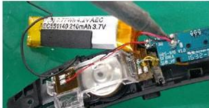
Remove battery wire.
