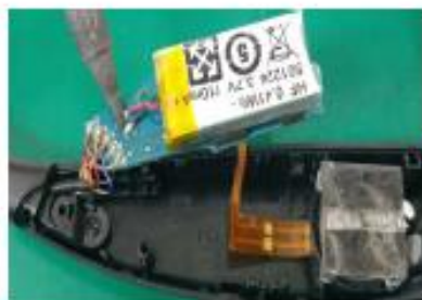
Remove battery wire.
