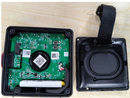
7.Remove the PR bracket.
