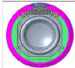
3) Disassemble of the Jersey Assy (2 screw)
