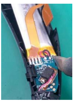
Remove battery wire.
