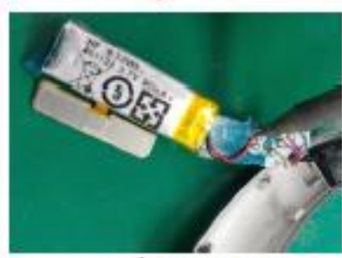
Remove battery wire.
