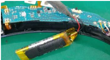
Remove battery wire.
