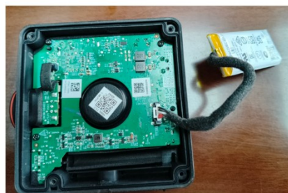
8. Remove the battery cable properly.
