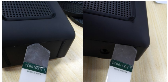
2. Insert the spudger into the pre-designed disassembly slot and pry upwards along the seam of the case in sequence (either clockwise or counterclockwise is acceptable).
