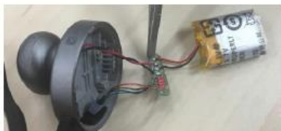
Remove battery wire.
