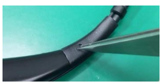
Remove screw cap.
