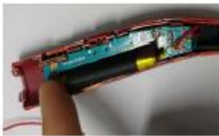
Detach battery from case.
