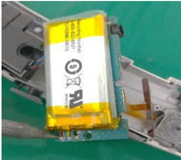
Remove battery wire.
