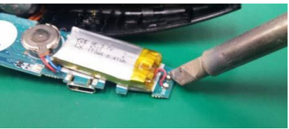
Remove battery wire.
