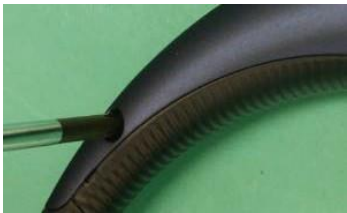
Remove screw (2point).
