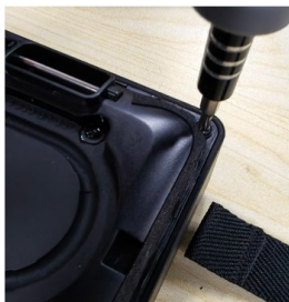
5. Sequentially remove the 4 screws that secure the PR bracket.
