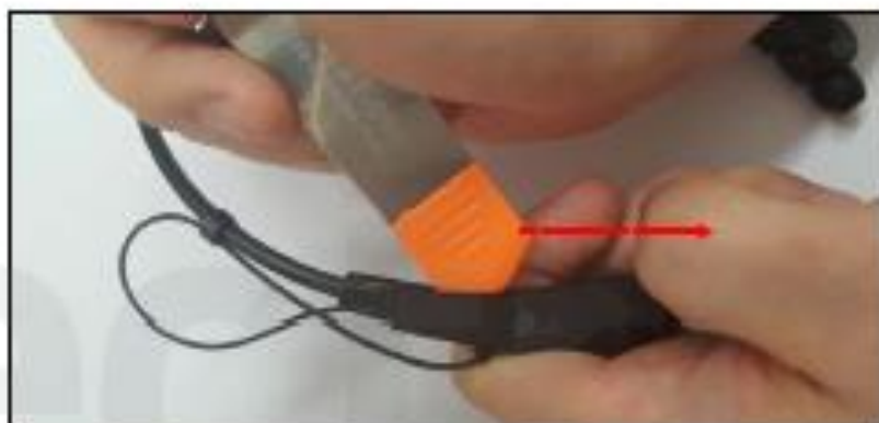
Insert the tool to the edge, and then disassemble from left to right.
