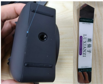
1. Prepare the spudgers for disassembly.
