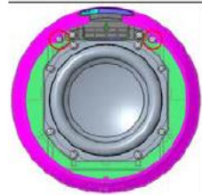
4) Disassemble of the Jersey Assy (2 screw)
