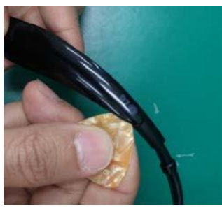
Insert the tool to the edge, and then disassemble right to left.
