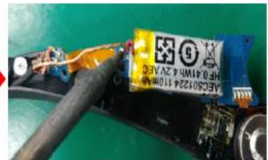
Remove battery wire.
