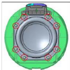
5) Disassemble of the WF Unit (8 screw)
