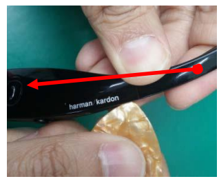
Insert the tool to the edge, and then disassemble from right to left..
