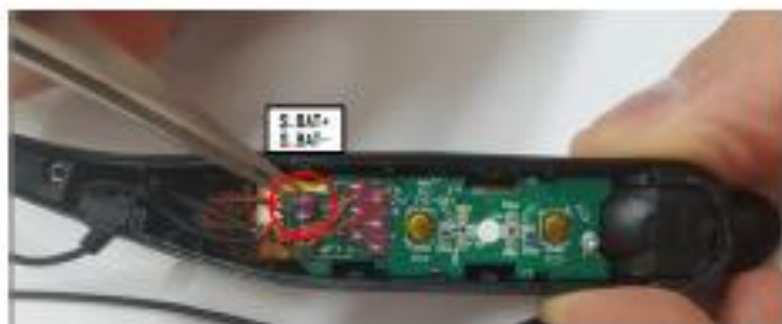
Remove UV bonding and remove battery wire.
