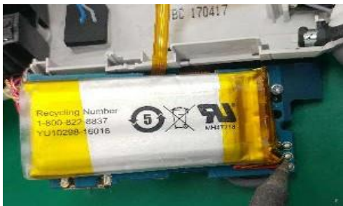
Remove battery wire.
