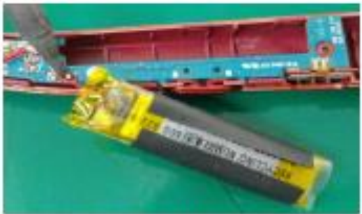
Remove battery wire.
