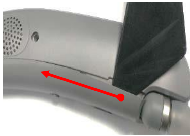
Insert the tool to the edge, and then disassemble from right to left.
