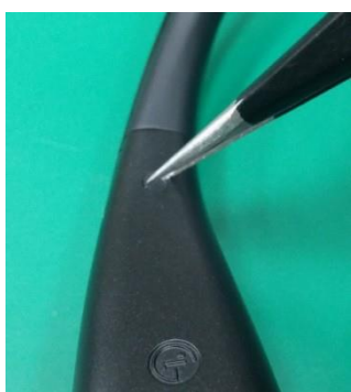
Remove screw cap.
