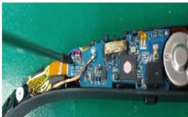
Remove screw (2point).
